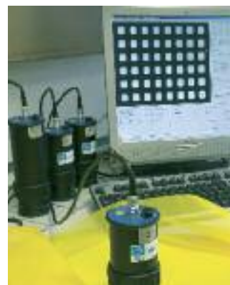
Measuring the thread count, mesh opening and thread diameter
